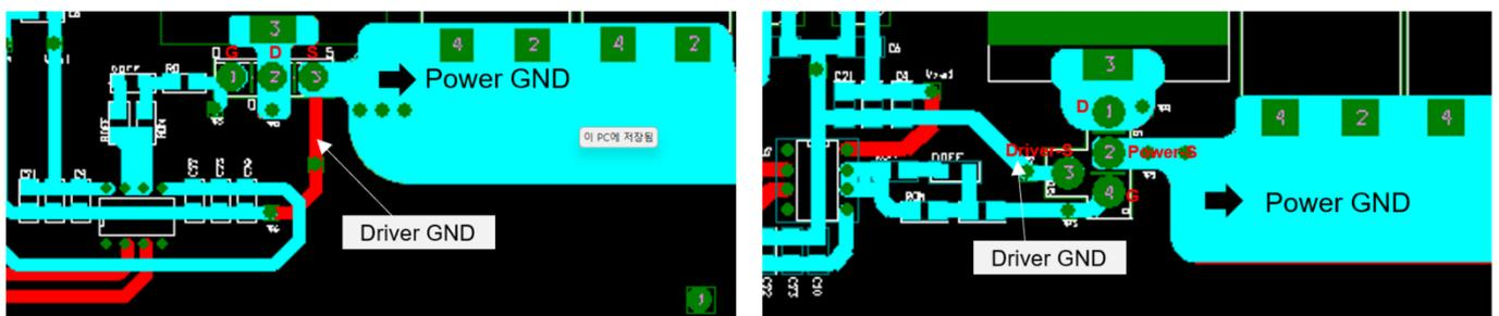
**Figure 4.** PCB Layout of Gate Driving Circuit : TO-247-3L (left) vs. TO-247-4L (right)
